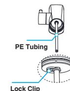
② Insert the PE Tubing (connecting the faucet and the pure water inlet of the water purifier, and the length is cut according to the actual situation) into the quick connector at the lower end of the faucet by about 16 mm, and then insert the lock clip (in the accessory package of whole machine) to prevent it from thread-off;
